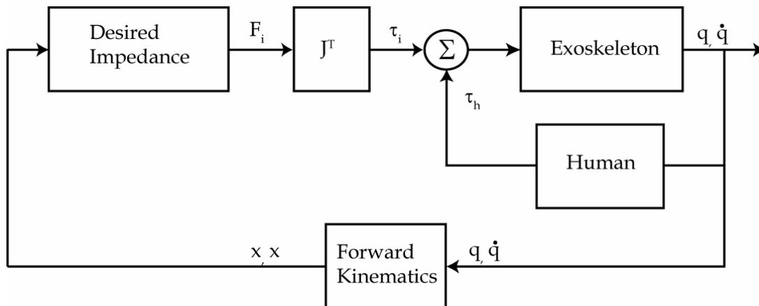
**Fig 10.** Task-space impedance controller for the MAHI arm exoskeleton, where,  $q$ ,  $q'$  are the current joint position and velocities;  $x$ ,  $x'$  are the current task-space position and velocities;  $F_i$  is the desired environment force;  $J$  is the Jacobian of the MAHI exoskeleton;  $\tau_i$  is the desired joint torques; and  $F_h$  is the human induced joint torque.
