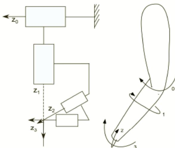
Fig 8. Simplified kinematic model of the human arm: Other axes have not been shown for clarity. Axes 0 through 3 represent elbow rotation, forearm rotation, wrist adduction/abduction and wrist flexion/extension respectively.
