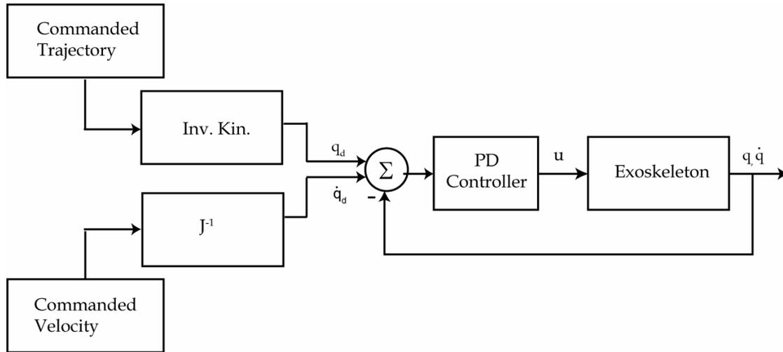
**Fig 9.** Inverse kinematics based trajectory controller for the MAHI Exoskeleton where,  $J$  is the Jacobian of the device;  $q_d$ ,  $q'_d$  are the desired joint position and velocities;  $q$ ,  $q'$  are the current joint position and velocities; and  $u$  is the control input.
