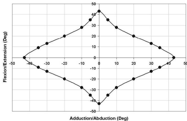
**Fig 6.** Range of motion of MAHI arm exoskeleton wrist
