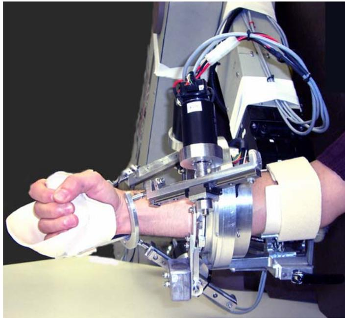
Fig 15. Subject operating the integrated MIME-RiceWrist System.
