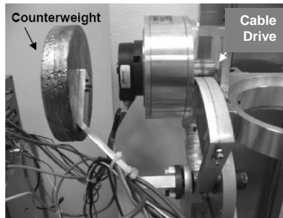
**Fig 3.** Elbow joint with a cable drive and counterweight for gravity compensation
