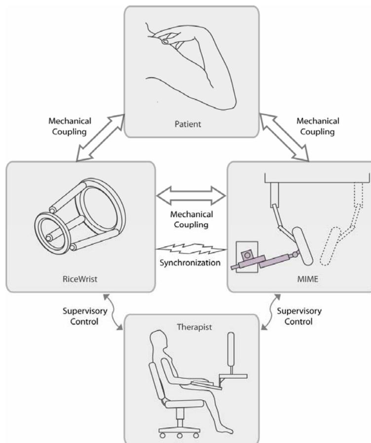
Fig 16. MIME-RiceWrist rehabilitation system setup
