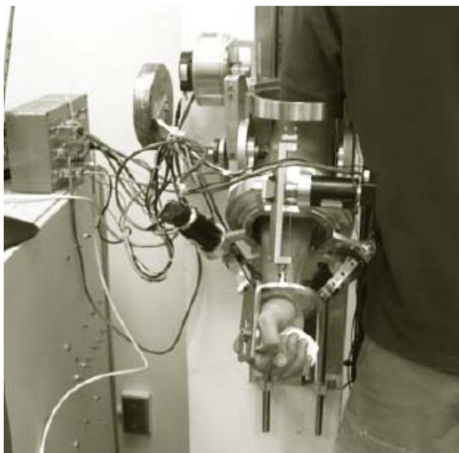
**Fig 5.** User operating the MAHI arm exoskeleton.
