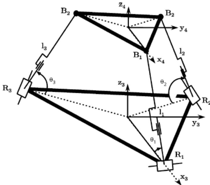
**Fig 2.** 3-RPS platform, adapted from (Lee and Shah 1988).
