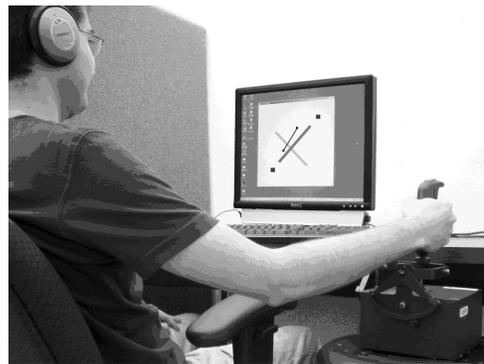
Figure 1: A participant is sitting at the training virtual environment. The interface includes a visual feedback display and a haptic joystick for force feedback, both of which provide feedback of the system dynamics to all trainees regardless of guidance scheme.
