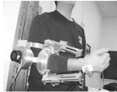
Fig. 1. User operating the exoskeleton.
