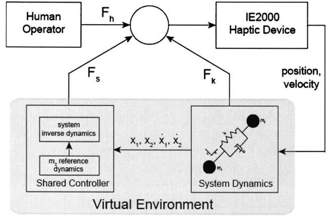
**Fig. 3 Block diagram of shared-controller architecture. The position and velocity of the joystick are mapped directly to that of  $m_1$ . The shared controller computes the force  $F_s$  (Eqs. (10) and (11)) that should act on  $m_1$  in order to follow the reference dynamics for  $m_2$ , as defined by Eqs. (8) and (9). The force  $F_s$  is reflected back through the haptic device in addition to the forces arising from system dynamics,  $F_k$  (Eqs. (5) and (6)).**
