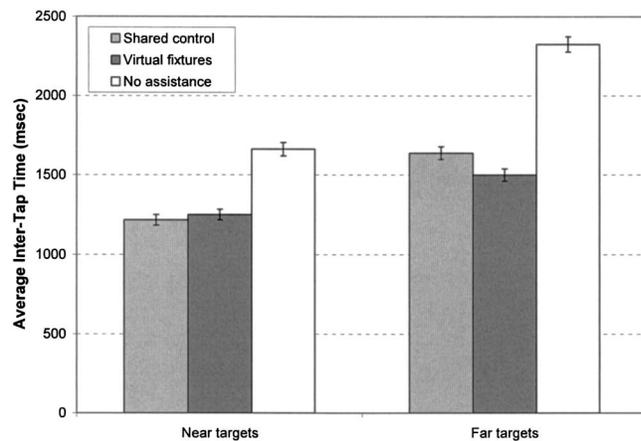
**Fig. 6** Experiment 1: Average time between target hits for performance assessment experiment. Shared control and assistance using virtual fixtures both provide significant and similar improvement in user performance as compared to the no-assistance case. A significant interaction was found between distance and assistance modes. The results for positive and negative sloped target pairs are combined in this figure.
