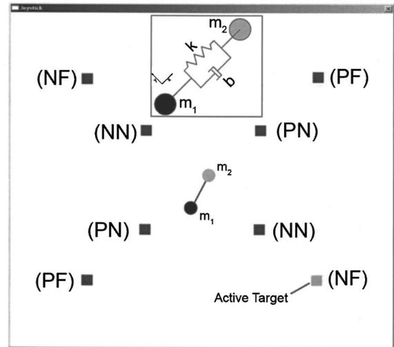
Fig. 2 Graphical display of tapping experiment. Subjects control location of  $m_1$  in order to cause  $m_2$  to hit the desired target. Targets appear in pairs (NF: negative slope, far; NN: negative slope, near; PF: positive slope, far; PN: positive slope, near). Inset shows virtual underactuated system. The user controls the system by applying forces to mass  $m_1$  through a joystick based interface.
