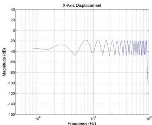
Figure 12: Typical X-axis displacement in a passive test
