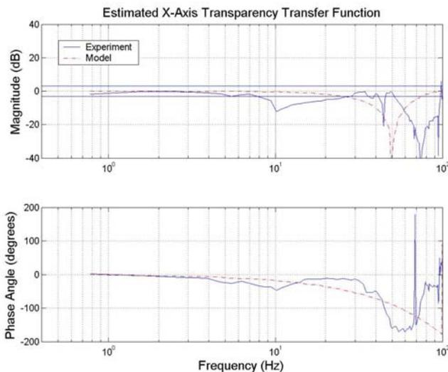
Figure 11: Typical estimated transparency of X-axis interaction in a passive test for measured and simulated manipulator dynamic forces
