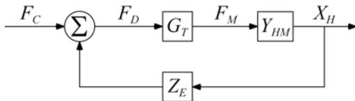
Figure 8: Block diagram of haptic interaction actively displaying force while user is a passive element
