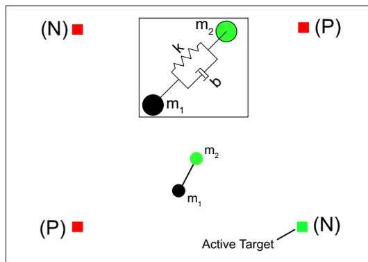
Figure 2: Graphical display of tapping experiment. Subjects control location of  $m_1$  in order to cause  $m_2$  to hit the desired target. Targets appear in pairs (N: negative slope; P: positive slope). Inset shows virtual underactuated system. The user controls the system by applying forces to mass  $m_1$  through a joystick based interface.
