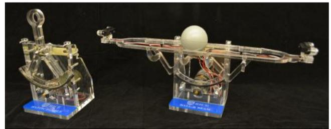
Figure 1. The “V3” Haptic Paddle and the Ball and Beam module at Rice University enable implementation in multiple courses and student experimentation in human visuo-motor learning experiments.
