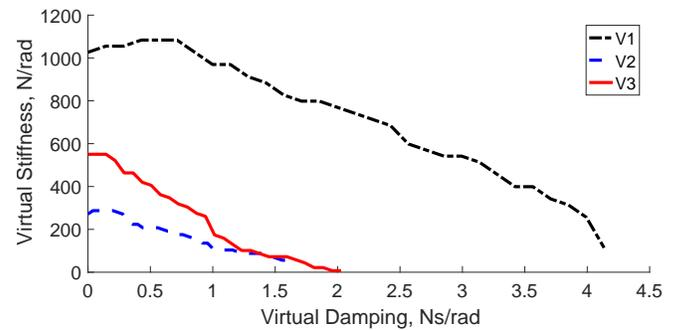
Figure 3. Z-width of the three versions of Haptic Paddles, “V1” [4], “V2” [5] and the new “V3”. While V1 possesses the largest Z-width, the friction drives of V2/V3 greatly increase device ‘up time’, with the improvement in V3 as a result of the friction transmission modifications.
