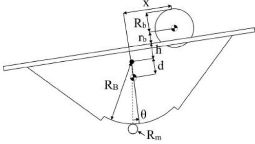
Figure 6. Simplified Haptic Ball and Beam schematic with parameters used to develop the virtual ball model.
