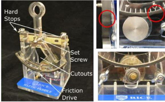
Figure 2. Haptic paddle design changes made to improve maintenance, assembly, and transmission performance (left). Specific changes to the friction drive including stiffer neoprene to reduce creep (circled in red) and higher speed reduction were made to improve haptic performance.
