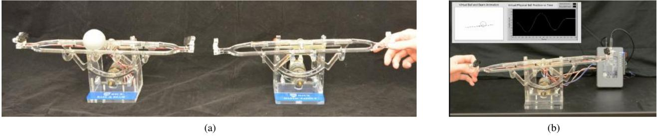
Figure 4. As shown in (a), students can teleoperate the ball and beam module, which provides a less abstract way to demonstrate principles of teleoperation. As shown in (b), students can also use the ball and beam module to render torques caused by a virtual ball in order to learn how haptic feedback can influence the learning of visuo-motor tasks by replicating experiments [14] or conducting new ones.
