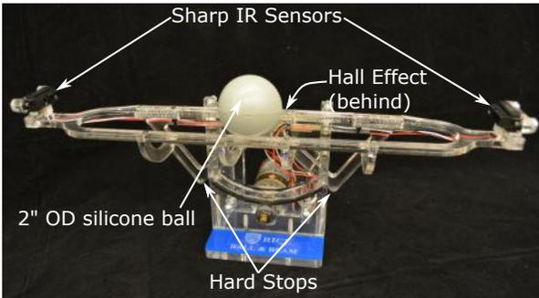
Figure 5. The Haptic Ball and Beam module, a low cost plant designed for bilateral teleoperation and visuo-motor human learning experiments. The ball position and beam angle is measured via two Sharp infrared (IR) sensors and a linear Hall-effect sensor, respectively.
