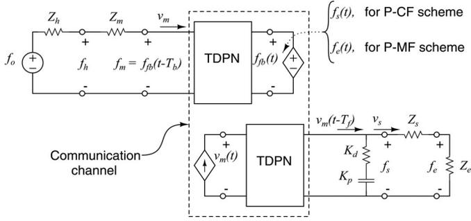
Fig. 3. Electrical network representation of P-F teleoperation schemes using TDPN formulation.
