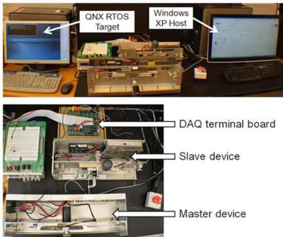
Fig. 11. Teleoperation experimental setup. Master and slave are linear, one DOF devices.
