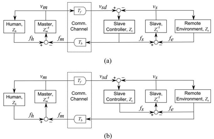
Fig. 2. Block diagrams representations of the position-force teleoperation schemes considered in this paper. (a) P-CF scheme. (b) P-MF scheme.
