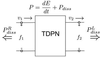
Fig. 4. Power flow in a TDPN. The power dissipated by the TDPN is divided into components observable at its left and right ports.
