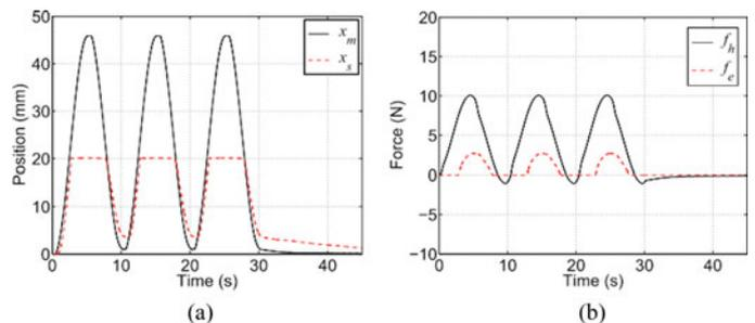
Fig. 10. Simulation results with the P-CF teleoperation scheme employing power-based TDPA with  $r$ -passivity. (a) Master and slave positions. (b) Operator and environment forces.
