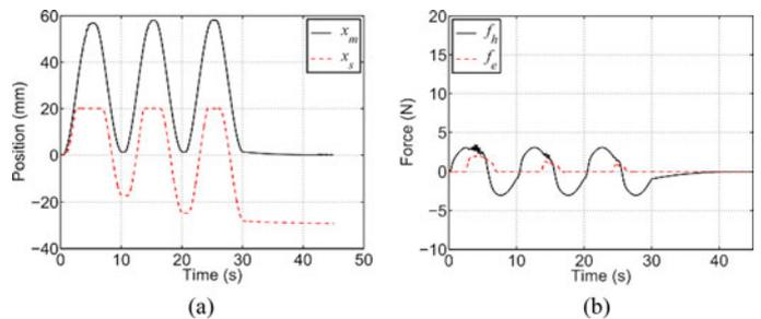
Fig. 9. Simulation results with the P-CF teleoperation scheme employing regular power-based TDPA. (a) Master and slave positions. (b) Operator and environment forces.
