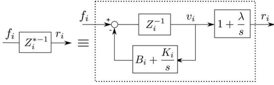
Fig. 7. Block diagram showing the devices augmented with a local FPC to passivate them with respect to  $r(t) = \dot{x}(t) + \lambda x(t)$ .
