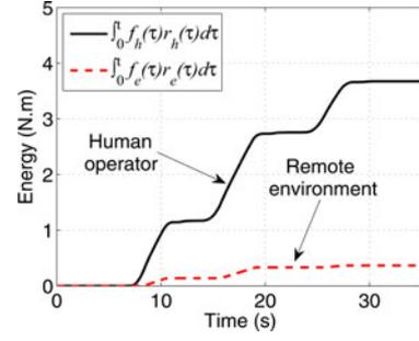
Fig. 8. Representative plot showing passivity of human operator and remote environment with respect to  $r_i(t) = \dot{x}_i(t) + \lambda x_i(t)$ . The operator force ( $f_h$ ) and environment force ( $f_e$ ) were measured to compute energy values.
