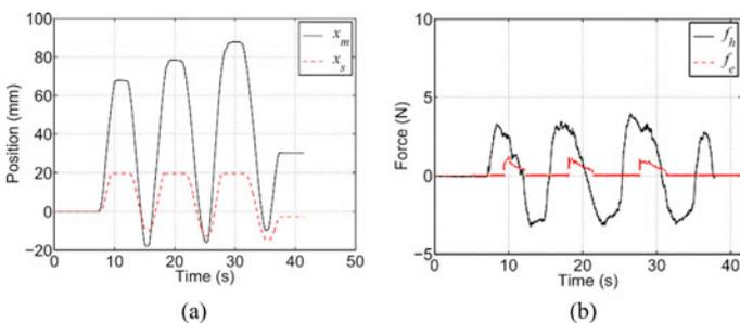
Fig. 12. Experimental results with P-MF teleoperation scheme employing regular power-based TDPA. (a) Master and slave positions. (b) Operator and environment forces.
