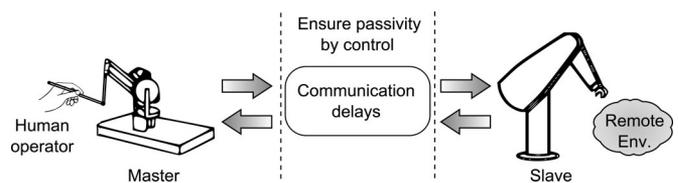
Fig. 1. Communication delays are the main source of activity in bilateral teleoperation. Passivity-based approaches aim to use control for passivating the communication channel, and hence ensure system passivity.
