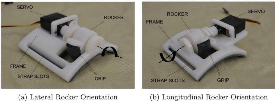
**Fig. 1.** The rocker is mounted in two orientations in order to compare user perception between the previously studied lateral orientation to the proposed longitudinal orientation.
