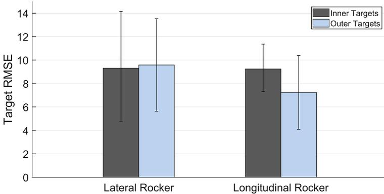
**Fig. 4.** The mean RMSE across all users for each experimental condition, error bars represent the RMSE standard deviation. The rocker orientation has a significant effect ( $p = .03$ ), where the lateral rocker has higher errors than the longitudinal rocker. In the longitudinal case, outer targets are easier to discern than the inner targets ( $p = .018$ ).
