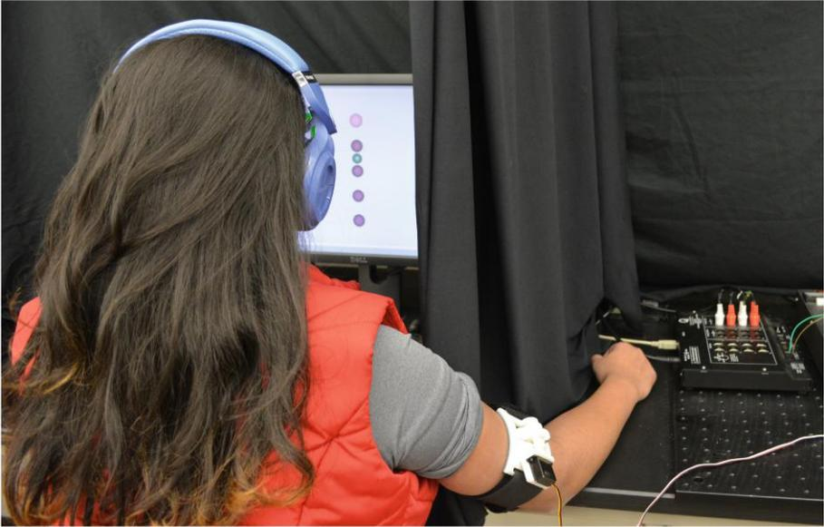
**Fig. 2.** The participant is seated at the bench facing the monitor, their right arm rests on the workbench with the rocker secured to the upper arm. Headphones provide pink noise to eliminate audio cues.
