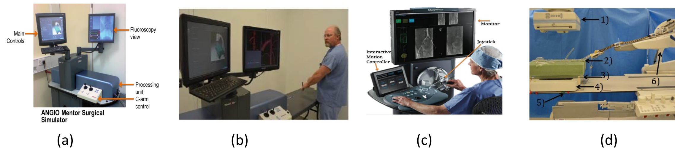
(a) 3D Systems VR platform (b) Subject cannulating VR model of vasculature (c) Subject manipulating RCM and surgical tools from Hansen Magellan remote workstation, (d) robotic system experimental set-up with 1) face of Siemens C-arm (for fluoroscopic images), 2) physical model, 3) Plexi-glass casing, 4) Window Field Generator for electromagnetic motion tracking, 5) Velcro straps, 6) Remote Catheter Manipulation (RCM) device.
