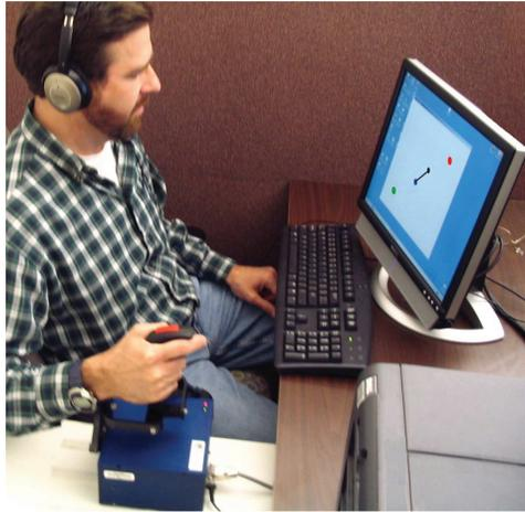
Fig. 3. Subject seated at the force feedback joystick, viewing the target-hitting task.
