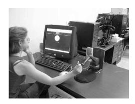
Fig. 1 User interacting with a webpage in which a haptic sphere has been embedded.
