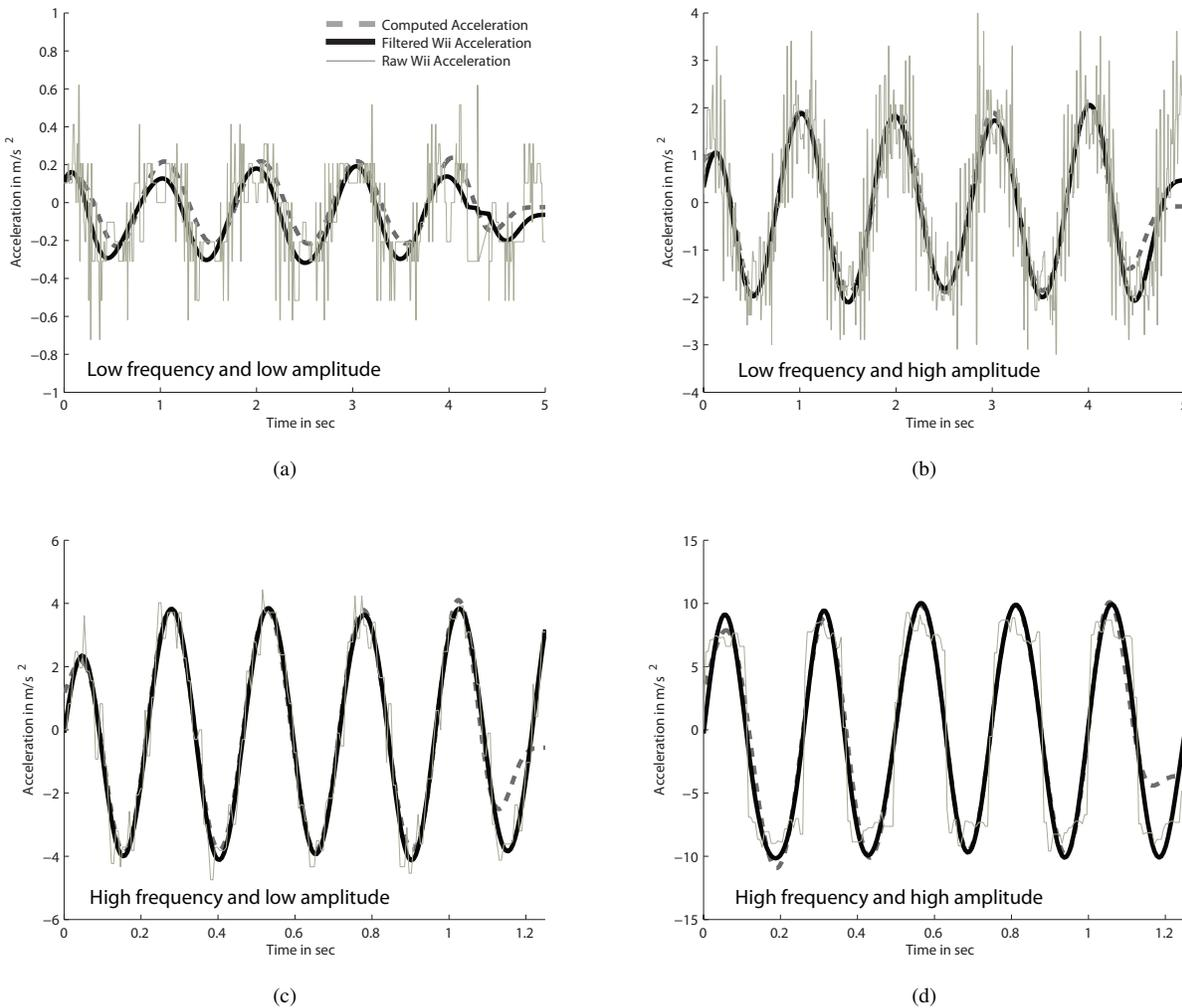
Fig. 3. Performance of the Wii's X-axis accelerometer at different frequencies and amplitudes, (a) 0.7 cm amplitude at 1 Hz, (b) 4.9 cm amplitude at 1 Hz, (c) 0.7 cm amplitude at 4 Hz, (d) 4.9 cm amplitude at 4 Hz
