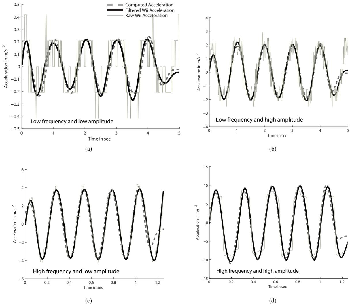
Fig. 5. Performance of the Wii's Z-axis accelerometer at different frequencies and amplitudes, (a) 0.7 cm amplitude at 1 Hz, (b) 4.9 cm amplitude at 1 Hz, (c) 0.7 cm amplitude at 4 Hz, (d) 4.9 cm amplitude at 4 Hz
