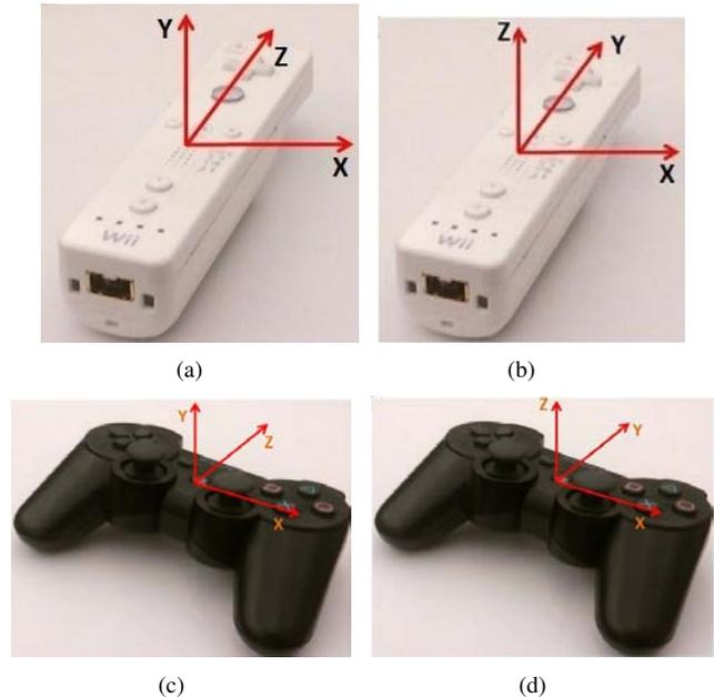
Fig. 1. (a),(c) show the coordinate system used by GlovePIE and (b), (d) show the local coordinate systems of the controllers
