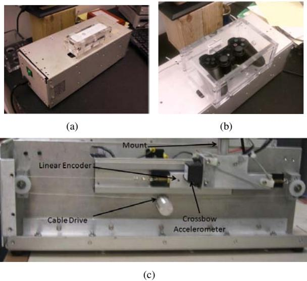
Fig. 2. One degree of freedom mechatronic test bed with (a) the Wii and (b) the Sixaxis controllers mounted for acceleration measurement comparisons. (c) Components of the one degree of freedom mechatronic testbed
