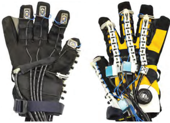
Fig. 7. The SeptaPose Assistive and Rehabilitative (SPAR) Glove with individually actuated thumb, index, and secondary fingers is a soft exoskeleton which relies on the wearer’s musculoskeletal system for reaction forces. This reliance on a wearer makes the SPAR Glove a good candidate for validation with the Instrumented Hand. Figure reproduced from [17].
