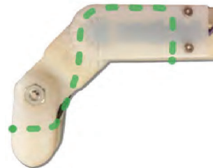
Fig. 3. Side view of the PIP and DIP joints on the instrumented hand show the 1:1 coupling achieved by using a Kevlar braided line (1 mm, Spear-It) as highlighted in green and anchored on either end.
