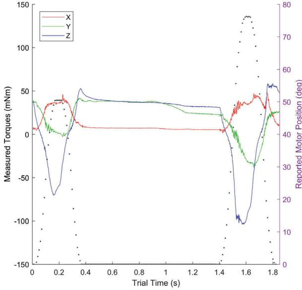
Fig. 5. Stretch module motor position in degrees overlaid onto x-, y- and z- axis torque outputs when stretch module is driven to 52°, back to 0°, waiting for 1 second then driving to 78° before finally returning to 0°. The force and torque data were reported from the sensors at 1000 Hz and the position data were reported from the motor controller at 100 Hz. Note that the PID controller operates at 2500 Hz; the 100 Hz reporting is due to hardware bandwidth limitations.
