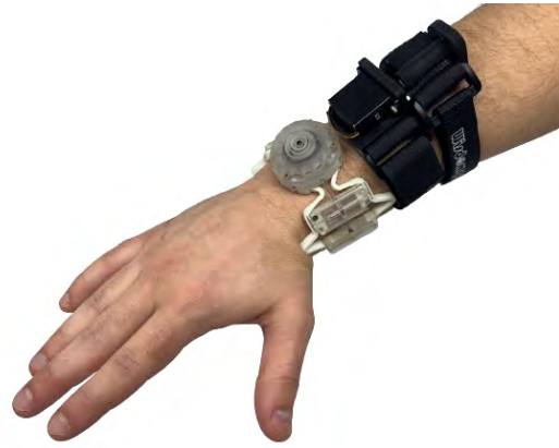
Fig. 1. MISSIVE-2 is a multi-sensory haptic wristband capable of delivering large sets of discrete haptic cues comprised of squeeze and vibration feedback. The vibrotactile band is positioned at the wrist, with the squeeze mechanism proximal to the vibrotactile band.
