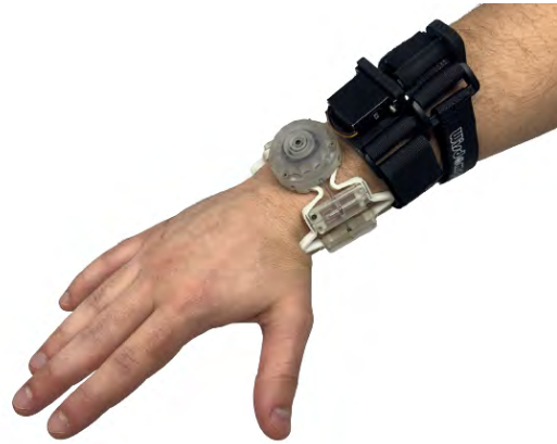
Fig. 1. MISSIVE-2 is a multi-sensory haptic wristband capable of delivering large sets of discrete haptic cues comprised of squeeze and vibration feedback. The vibrotactile band is positioned at the wrist, with the squeeze mechanism proximal to the vibrotactile band.
