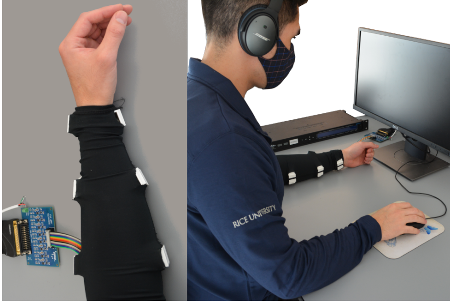
Fig. 1. Participant wearing the vibrotactile sleeve, positioned to complete the experimental task. (left) Vibrotactile sleeve used in experiments to deliver vibrotactile cues to the participant via 6 vibrotactors. Tactors were evenly spaced on the participant’s forearm between their wrist and elbow with 3 vibrotactors on the ventral side of the arm and 3 vibrotactors on the dorsal side. (right) Participant wearing the vibrotactile sleeve while interacting with the experimental GUI on the monitor and listening to pink noise through headphones.
