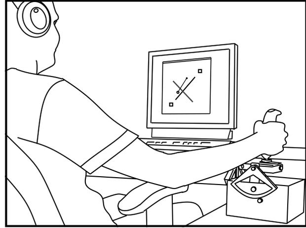
Figure 1: A participant is sitting at the virtual training environment. The interface includes a visual feedback display and a haptic joystick for force feedback, both of which provide feedback of the system dynamics to all trainees regardless of guidance scheme.
