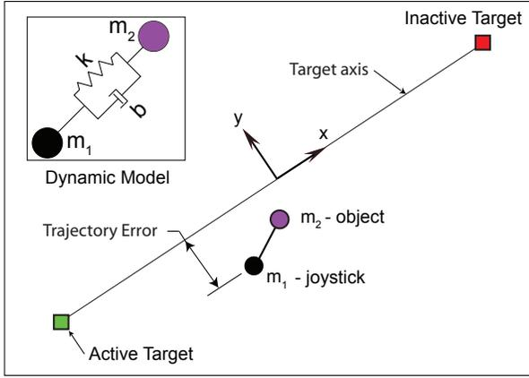
Figure 2: Target hitting task: the participant controls the location of  $m_1$  (force feedback joystick) in order to cause  $m_2$  (object) to hit the active target. Inset shows the virtual underactuated system. Trajectory error is defined as the deviation of  $m_1$  (object) from the target axis (adapted from [15]).
