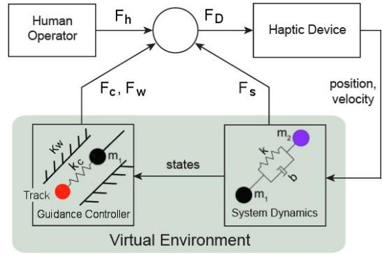
Figure 5: Block diagram of the haptics-enabled virtual training environment with haptic guidance augmentation. The guidance is in the form of virtual walls to mitigate deviation from the target axis and in the form of a PD tracking controller to encourage excitation at the resonant frequency of the system.
