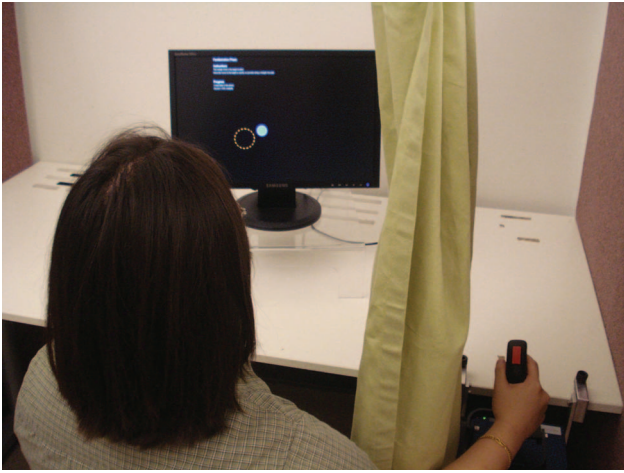
Fig. 1. Setup used for the experiment. Participants were seated in front of a computer monitor and moved an Immersion IE2000 joystick with their dominant hand. A curtain obscured the joystick and the controlling hand from view. Note objects on the screen have been enlarged for greater visibility.
