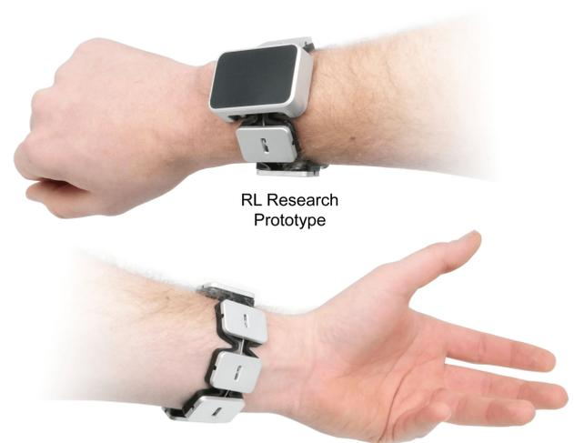
Fig. 1. Tasbi is a compact multimodal haptic wristband capable of delivering vibrotactile feedback at six locations and uniform squeeze feedback around the wrist (tethering cable not shown).
