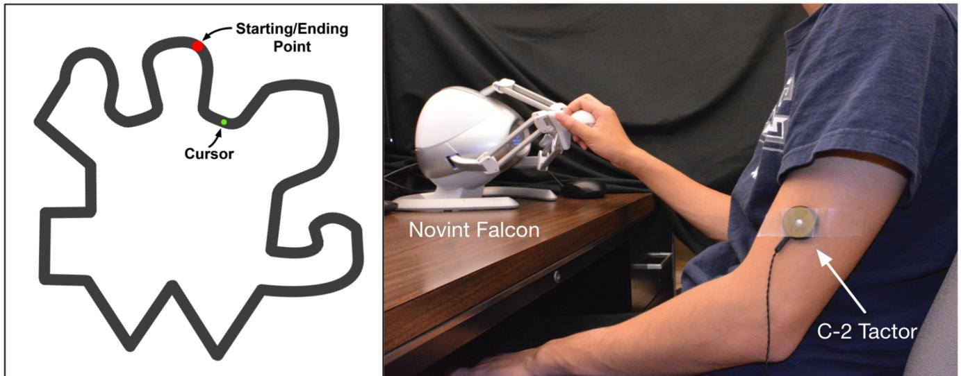
Fig. 1. The subject navigates the cursor around the abstract shape using a Novint Falcon as the input device. In the mirror-tracing task, the movements of the input device are inverted compared to the movements of the cursor on the screen. Tactile feedback of performance is provided by a C-2 tactor secured to the subject's non-dominant arm.
