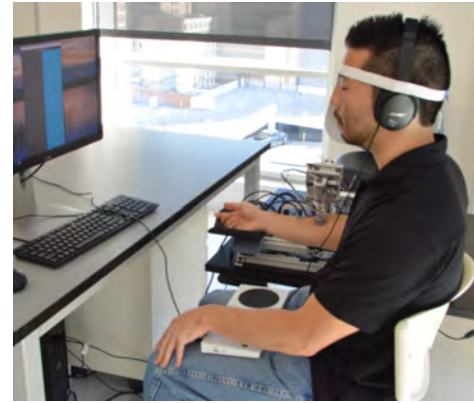
Fig. 4. The user is seated in front of a monitor with their right arm in the test bed, adjusted according to their comfort. Headphones playing pink noise mask any audible noise from the test bed's motors. The user interface sits either on the table in front of them or on their lap, according to their preference.
