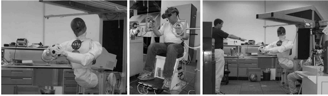
Figure 4 Robonaut holding ball, teleoperator driving Robonaut, and task leader gesturing the desired location of the ball
