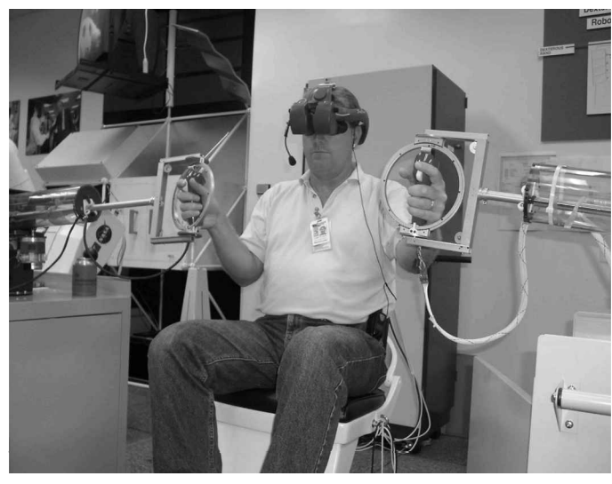
Figure 2 The teleoperation interface used in the assembly task trials with kinesthetic feedback
