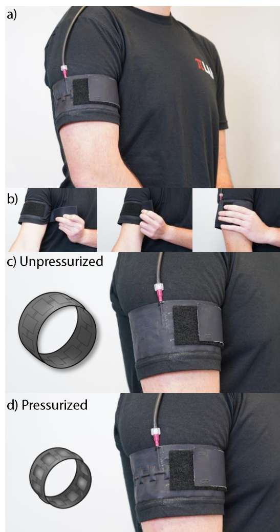
Figure 6. Seamless integration of a textile-based haptic device into a garment. (a) Shirt with a squeeze-enabled haptic device permanently heat sealed onto the sleeve. (b) Hook and loop fastening method to tighten the sleeve around the arm for a salient cue. (c) Unpressurized squeeze band on arm. (d) Squeeze cue delivered through application of pressurized air.
