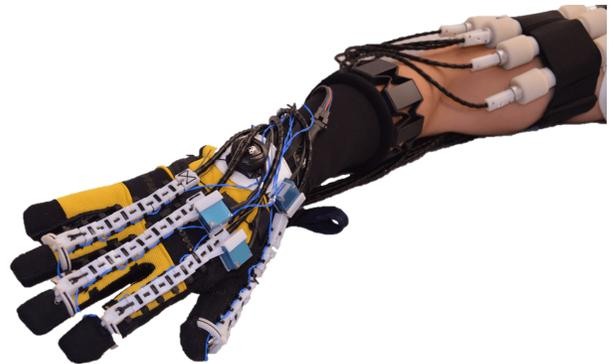
Fig. 2. The SPAR Glove combines a novel glove-based exoskeleton with intent detection at the wrist, EMG at the forearm, and proximally located actuation to create a powerful, wearable system for hand assistance and functional task based training. Motors can be packaged in a wide range of configurations on the arm or in a backpack.
