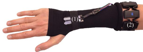
Fig. 7. The intent detection subsystem of the SPAR Glove consists of flexible resistors (1) located at the wrist for measuring the tenodesis grasp, and the Myo armband (2) for EMG detection.
