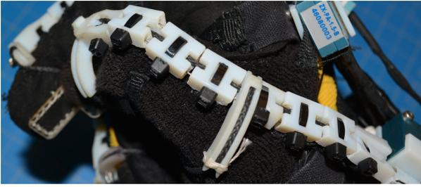
Fig. 5. Hyperextension vertebrae are segmented links, connected to the glove with either a whipstitch or zip tie (zip tie pictured here for the thumb). The vertebrae are 0.5" long and 0.4" and use a thin steel cable routed alongside the kevlar tendon to maintain alignment.
