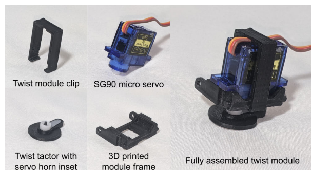
Fig. 3. The twist module with base components. The twist module clip holds the micro servo motor to the twist module frame. The micro servo motor provides the twist actuation through the example twist factor to the skin. Designers can customize the twist factor shape and apply various materials to interface between the factor and the skin.
