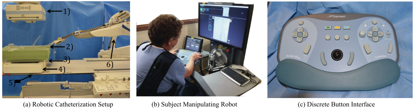
Fig. 2. (a) Magellan setup, with 1) the face of the Siemens C-arm to generate fluoroscopic images, 2) Fundamentals of Endovascular Skills (FEVS) model with styrafoam housing, 3) plexi-glass casing, 4) Window Field Generator, 5) velcro straps to secure setup to patient table, and 6) Remote Catheter Manipulation (RCM) device. (b) Subject manipulating the RCM and surgical tools from the remote workstation. (c) Button interface to control Magellan tools.
