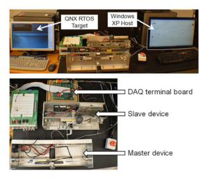
Fig. 11. Teleoperation experimental setup. Master and slave are linear, one DOF devices.
