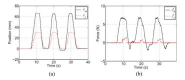
Fig. 13. Experimental results with P-MF teleoperation scheme employing power-based TDPA with r-passivity. (a) Master and slave positions. (b) Operator and environment forces.
