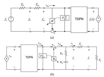
Fig. 5. Passivated TDPN with the PO/PC. Note that the PC is not required on the ports connected to the ideal sources. (a) PO/PC in impedance configuration. (b) PO/PC in admittance configuration.
