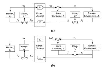
Fig. 2. Block diagrams representations of the position-force teleoperation schemes considered in this paper. (a) P-CF scheme. (b) P-MF scheme.
