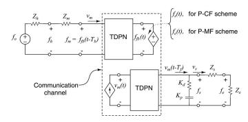
Fig. 3. Electrical network representation of P-F teleoperation schemes using TDPN formulation.
