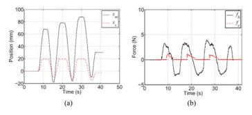
Fig. 12. Experimental results with P-MF teleoperation scheme employing regular power-based TDPA. (a) Master and slave positions. (b) Operator and environment forces.
