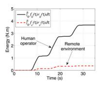
Fig. 8. Representative plot showing passivity of human operator and remote environment with respect to  $r_i(t) = \dot{x}_i(t) + \lambda x_i(t)$ . The operator force  $(f_h)$  and environment force  $(f_e)$  were measured to compute energy values.
