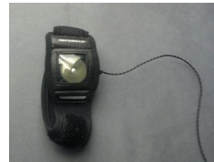
Figure 5. The armband used to attach the tactor to the subject. This secured the tactor against the subject's bicep.
