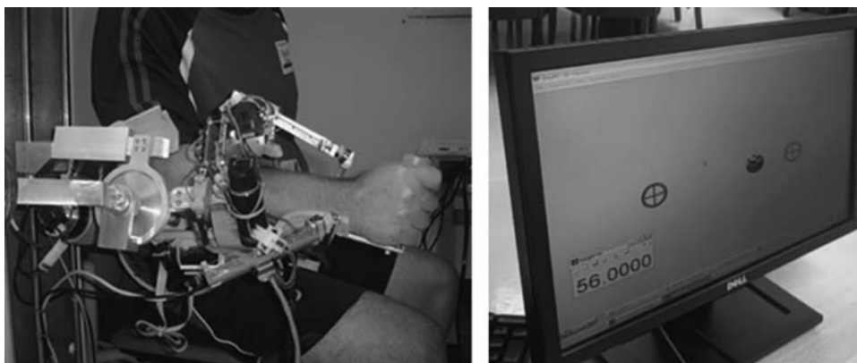
FIGURE 1. MAHI Exo-II robotic device during training (left) and target hitting task (right).
