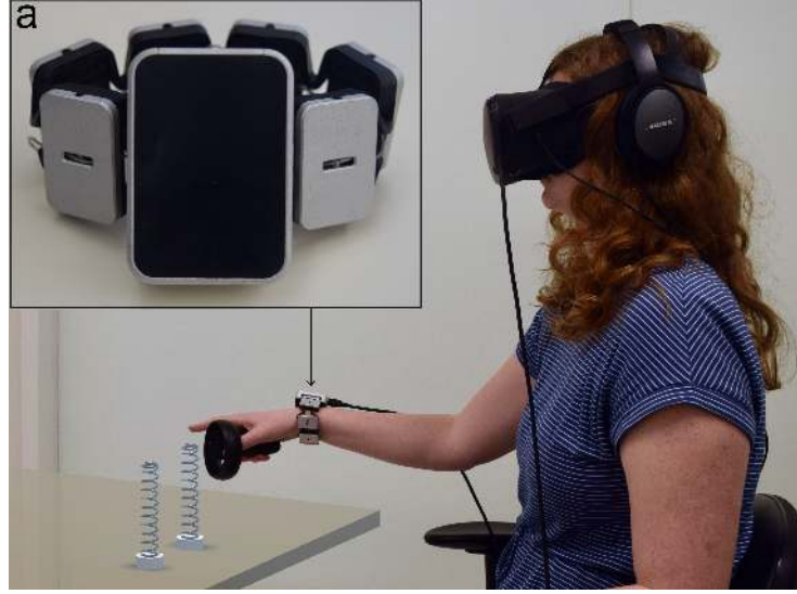
Fig. 1. Study Setup: A participant is seated with no obstruction to movement. They see two virtual springs in front of them. They have the Tasbi haptic device (a) tightened onto their right wrist, an Oculus controller in their right hand, an Oculus headset on their head, and noise-canceling over-ear headphones.
