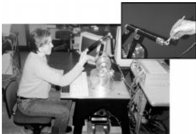
Fig. 1. Test subject seated at haptic interface holding stylus with dominant hand. Insert shows close-up of stylus and recommended handgrip.
