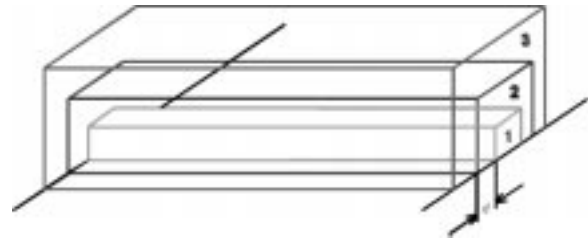
Fig. 4. Representation of square cross-section ridges in three rendered sizes showing ridge size difference, d .
