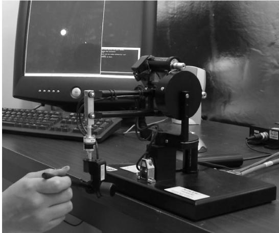
**Figure 4. PHANToM Premium 1.0A with load cell for force measurements.**
