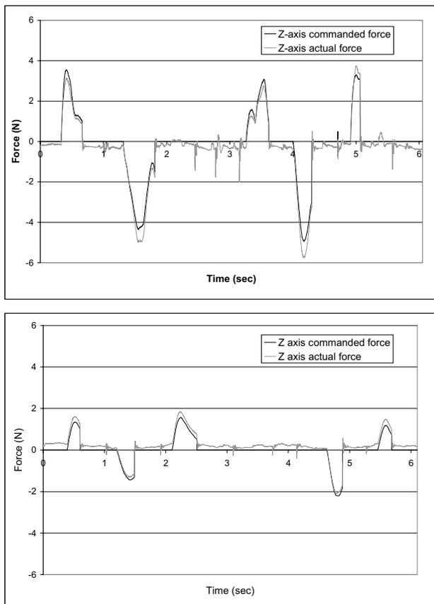
**Figure 5. (top) Unsaturated case (bottom) Saturated (2.2 N) and limited stiffness (220 N/m) case**
