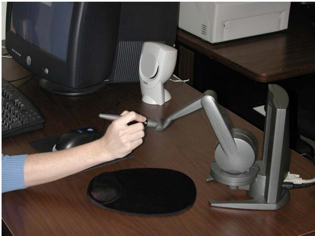
**Figure 2. Test subject seated at testing station for virtual environment experiments. (The curtain used to obstruct the subject's view are removed in this picture)**
