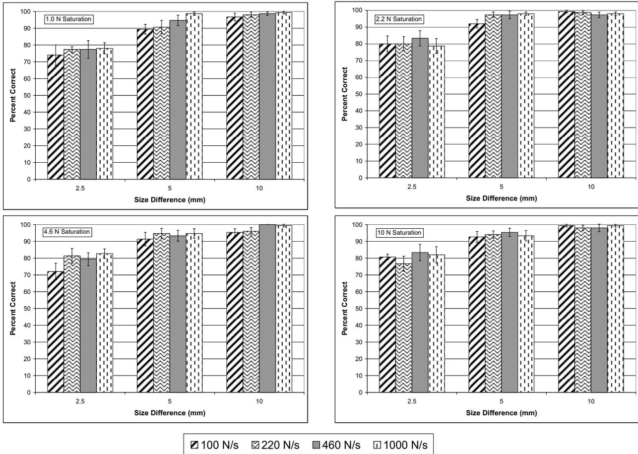
Figure 3. Results for size discrimination experiments for all force saturation values tested: 1 N (upper left), 2.2 N (upper right), 4.6 N (lower left), 10 N (lower right).
